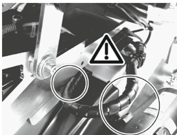
Lifter column completely retracted. Pay attention to areas where the cable bundle might get crushed or touch the motor.
