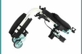
Compact size (765x390x285 mm): fold the wheelchair and its backrest, remove the rear wheels, and it fits in the smallest of cars.
